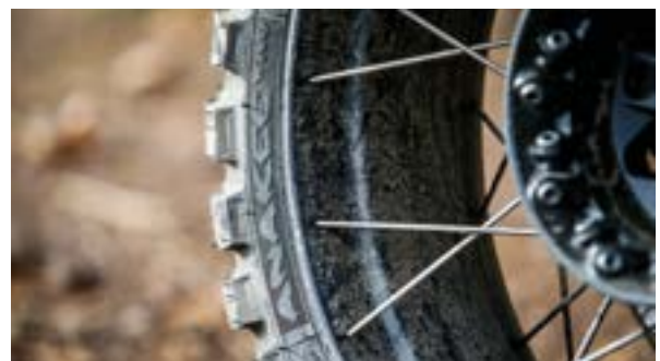
A spoke rim that is Tubeless (TL): the spokes are fixed on the edges maintaining the seal.
